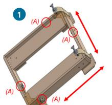
Loosen the four wing nuts (A) on the sides of the Raiser and expand it out to the approximate size of the base of the chair.
