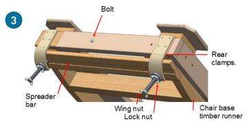
Clamp the raiser to the chair by placing the spreader bar over the timber runner of the chair base and tightening the rear clamps down onto the spreader bar. Tighten the lock nut.
