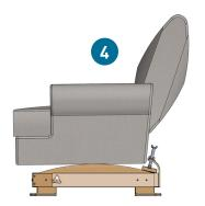
Carefully place chair upright. Check that all runners of the chair are positioned safely in the corners of the raiser. Sit on the raised chair and check that it feels safe. The raiser is now fitted and ready for use.
