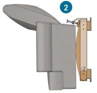
Roll the chair forward so the feet of the chair are accessible. Adjust the Raiser so the lip of the Raiser fits snugly over the base of the chair. Tighten the 4 x wing nuts firmly.
