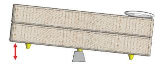
Remove the Multifit Bedjack. Place a weight at the foot end of the bed. This will cause the head end of the bed to rise. Place bed blocks under the legs at the head of the bed.
