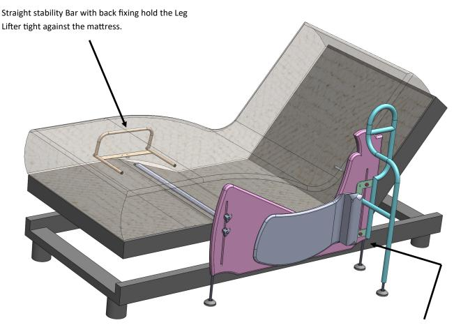
The other end of the Leg Lifter will need to be fixed to the base frame of the bed with a cord.
