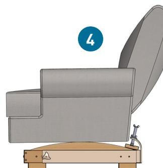
Carefully place chair upright. Check that all runners of the chair are positioned safely in the corners of the raiser. Sit on the raised chair and check that it feels safe. The raiser is now fitted and ready for use.
