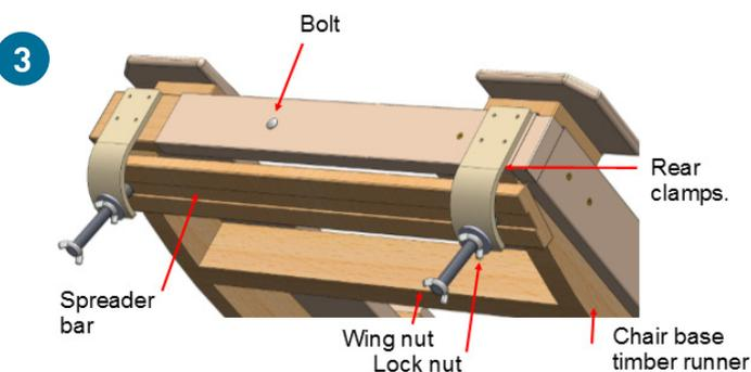
Clamp the raiser to the chair by placing the spreader bar over the timber runner of the chair base and tightening the rear clamps down onto the spreader bar. Tighten the lock nut.
