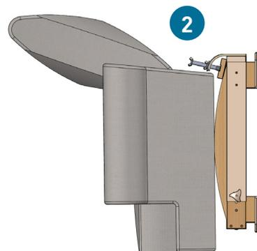
Roll the chair forward so the feet of the chair are accessible. Adjust the Raiser so the lip of the Raiser fits snugly over the base of the chair. Tighten the 4 x wing nuts firmly.
