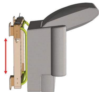
**3** Thread the cord up and around the round steel tube then down into the cleat. Lastly pull the cord upward and into the V of the cleat to clamp the cord in place.
