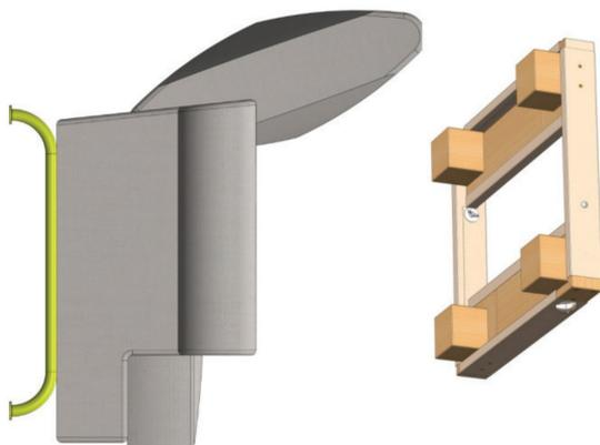
**2** Adjust the Raiser so the lip of the Raiser fits snugly over the base of the chair. Tighten the 4 x wing nuts firmly.
