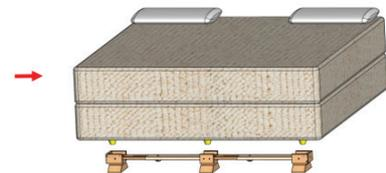
**3** With the Multifit Bed Jack raise the end of the bed. Place the Bed Raiser under the center legs. Lower and remove the Jack.
