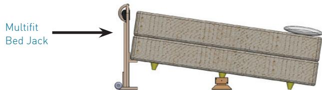
**4** Put a weight on the foot end of the bed (anything 3-5kg will do). Place a raiser under the head end. Remove the weight.
