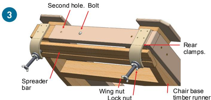
Clamp the raiser to the chair by placing the spreader bar over the timber runner of the chair base and tightening the rear clamps down onto the spreader bar. Tighten the lock nut.
