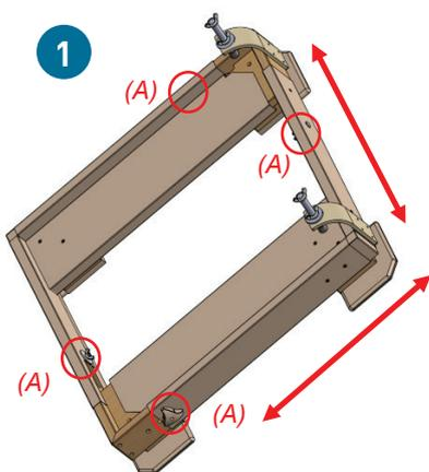
Loosen the four wing nuts (A) on the sides of the Raiser and expand it out to the approximate size of the base of the chair.
