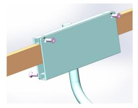
Repeat the clamping procedure with the far side clamp plates.
