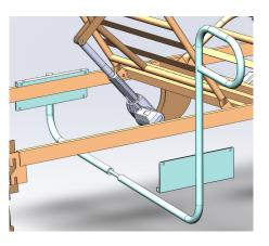
Position the far end of the rail so it rests on the far side rail of the bed frame.
