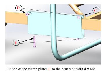
countersunk head Allen key drive bolts D
