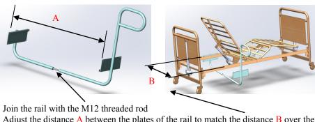
Adjust the distance A between the plates of the rail to match the distance B over the side rails of the bed frame.
