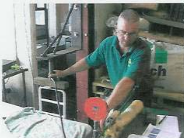
Here downward pressure of 750 Newton's is put on the end of the rail. That's approx equal to the force required to lift 75KG.
