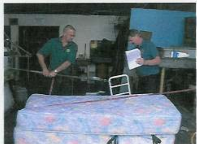
Here lateral force of 50 Newton's is pulled from the side of the rail. That's approx equal to the force required to lift 50KG.
