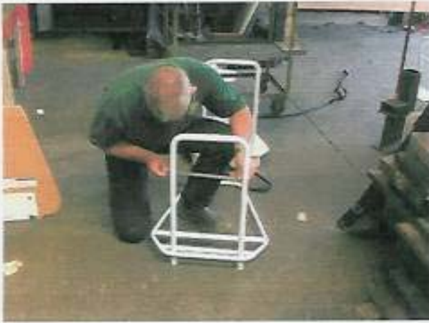
Measuring the opening sizes to see that the distance between the upright tubes is more than 250 mm.
