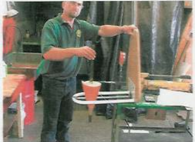
Here Jim is inserting a cone of specific size and shape into the gap between the bars of the Safety rail.
